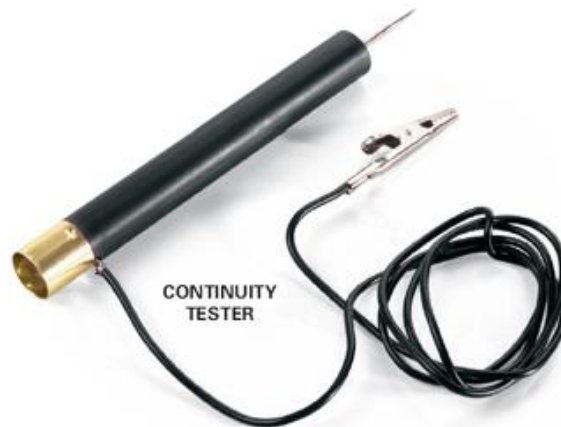
Figure 1: A Simple Continuity Tester
